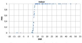
Fig. 1. PRR/SNR curve for an indoor environment.
