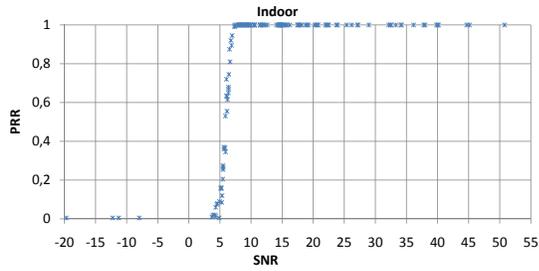
Fig. 1.  $PRR/SNR$  curve for an indoor environment.
