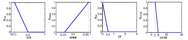
Fig. 2. Definition of membership functions. For instance, for  $\mu_{SPRR}$ , for values of  $SPRR$  below 25%, the link is considered totally out of the fuzzy subset of links with high  $PRR$ . Starting from 95%, the membership to the fuzzy subset of links with high  $PRR$  is of 1. For values of  $SPRR$  between 25% and 95%, the membership increases linearly from 0 to 1.
